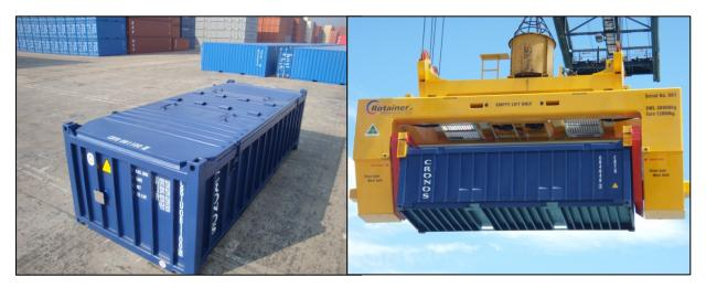
The rotating device is attached to a portainer with standard equipment. Portainers with rotating devices fitted are able to lift the purpose built containers and lower the container deep into the cargo hold of a ship and then rotates the container until all the material inside the container has been emptied into the hold.
